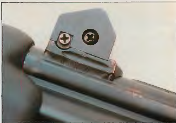
Housing a rugged ghost ring, XS Sight Systems' HK Rear Sight is rugged and fully adjustable. Note the marred finish on this well-used MP5 before it was redone.
